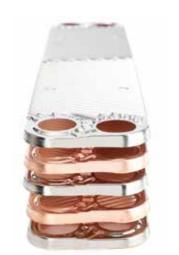
A brazed plate heat exchanger (BHE) is very compact compared to other heat exchangers for similar applications, meaning less refrigerant is needed. AlfaNova is a range of fusion-bonded, all-stainless-steel heat exchangers. They are ideal in situations involving media that is corrosive or very sensitive to contamination of copper or nickel.
